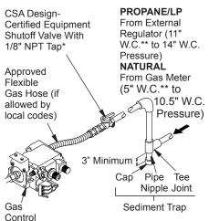
Figure 16 - Gas Connection (Remote-Ready Models Only)
